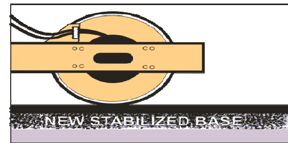
Pave with new asphalt course and roll
