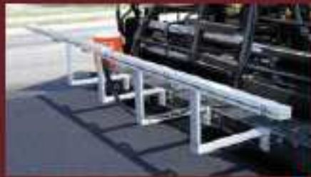
Temp sensor bar on paver (TX Transportation Institute Prototype)
